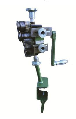
The Tin Knocker 2n1 Crimper Beader is a machine that is light weight and can perform both beading and crimping. This manual hand cranked machine is portable and works great in the field for the insulation trade where light gauge materials are used.
